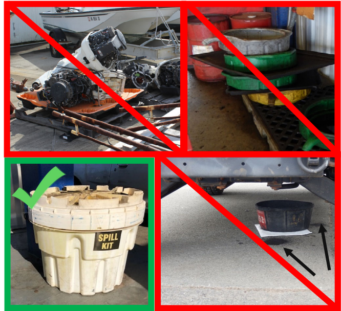
Photos: (Top Left) Used parts improperly stored outside without adequate cover & containment. (Top Right) Used drip pans stacked over edge of spill pallet. (Bottom Left) Clearly labelled & accessible spill kit near work area. (Bottom Right) Improper placement of drip pan & absorbent.
