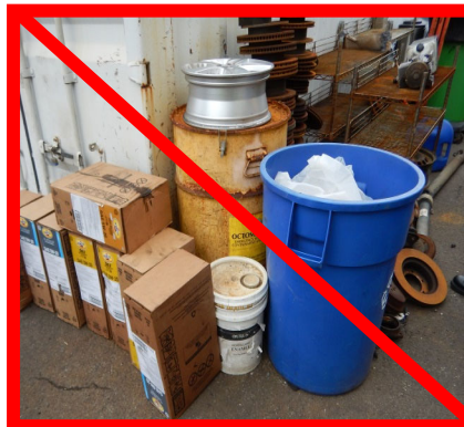
Photos: (Left) Containers of auto fluids, rusted drum & car parts stored outside without cover or spill pallet. (Right) Proper BMPs for transferring waste to drum (i.e. funnel & absorbent).
