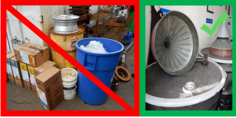
Photos: (Left) Containers of auto fluids, rusted drum & car parts stored outside without cover or spill pallet. (Right) Proper BMPs for transferring waste to drum (i.e. funnel & absorbent).
